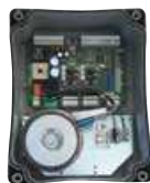
T624 Central de control
